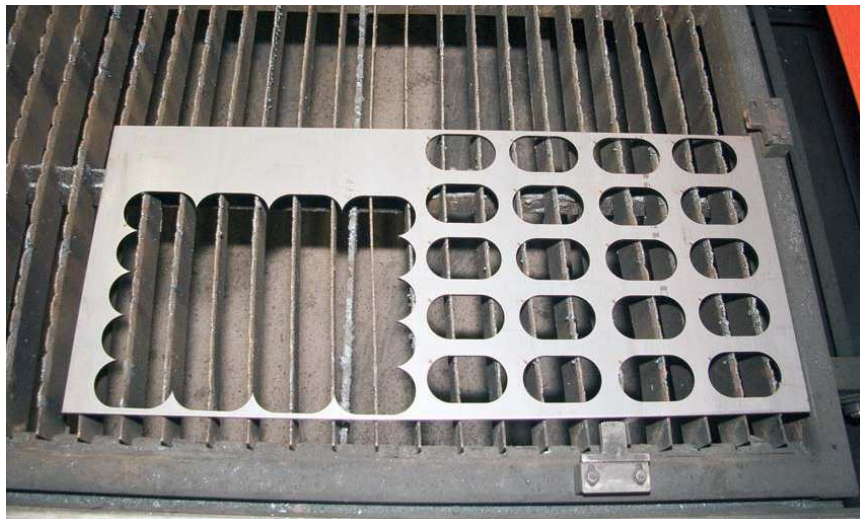
Fig. 2. Tomologic’s technology (left) compared to the traditional nesting technology (right).
